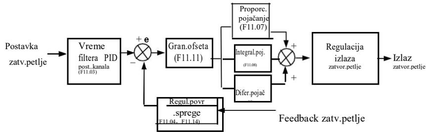
**Fig.7-37 Princip rada PID regulatora**
