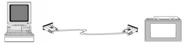
Before user download a program, please make sure your PC has installed multiport serial card or USB-RS232 convertor, and connect cable correctly, click "" button in Touchwin software, then you could download data successfully, below are the pin definitions:
